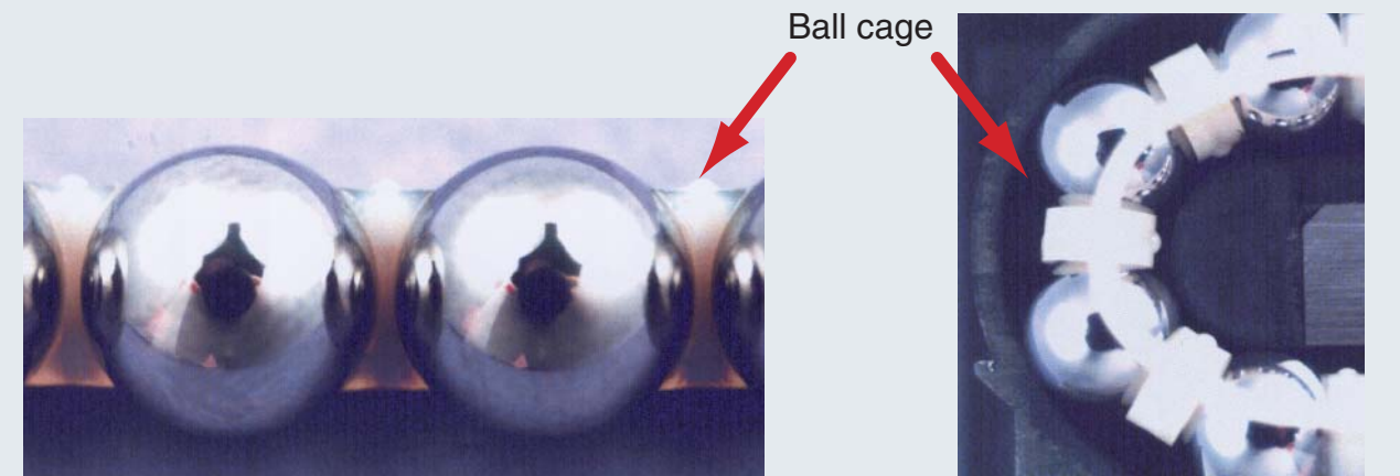
Contact state between balls and ball cage
